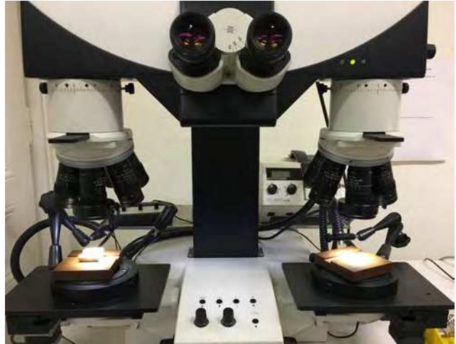
Figure 2: Leica comparison microscope which is used for capturing the toolmark images.
