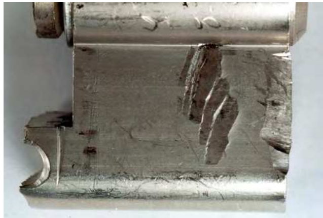
Figure 1: Snapped lock cylinder with the broken mounting highlighted on the left and the toolmarks on the right.
