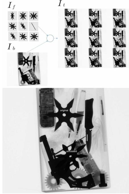
Figure 11. Simulation of a shuriken superimposed onto an X-ray image of a bag. The original X-ray image ( $I_b$ ) has only one shuriken, whereas the simulated X-ray image ( $I_t$ ) has an additional shuriken in different poses (see the shuriken partial occluded by the gun). Bottom image shows a zoom in of a simulated image.
