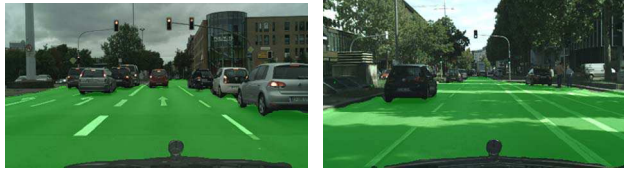
Figure 2: Output of the road labeling network. With green the detected road is marked in the image.
