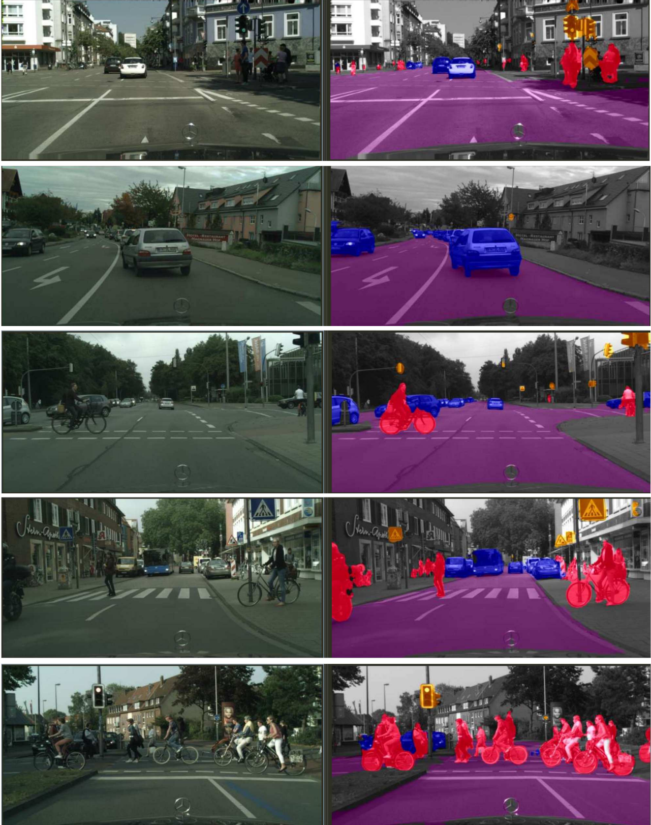
Figure 3. Sample input images from the validation set and the segmentation produced using sparse (80%), quantized inference (chroma blended visualization)
