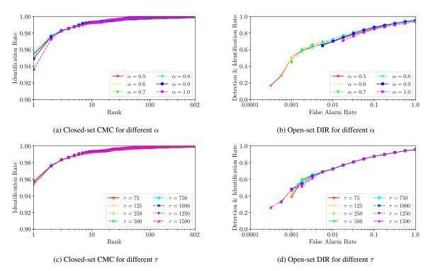
Figure 2: EVM HYPERPARAMETER SELECTION. Two different parameters of EVM are optimized: the distance multiplier  $\alpha$  and the tail size  $\tau$ . Both are evaluated using the CMC curve on probe set C and the DIR curve on probe set  $O_3$ .
