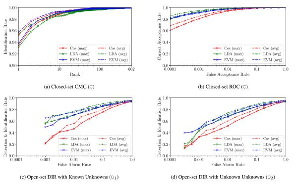
Figure 3: COMPARISON BETWEEN METHODS. The (a) CMC curves and the (b) ROC curves for the closed-set evaluation on probe set C, as well as the open-set DIR curves for (c) probe set  $O_1$  and (d) probe set  $O_2$  are given for all six evaluated methods.
