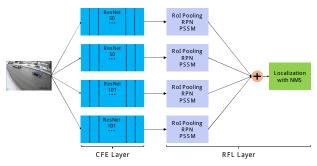
Figure 4. An illustration of the multi-network ensemble for region-based object detector. For the an input data, each model generates candidate boxes through the CFE and RFL layers, and then the generated boxes are merged into an image by NMS.
