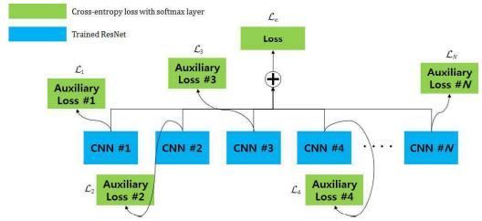
Figure 1. A conceptual sketch of JF for the model ensemble. Outputs of all CNNs are element-wise added, and they are used for the final prediction. Each CNN has an auxiliary loss for preventing loss of previously learned information.
