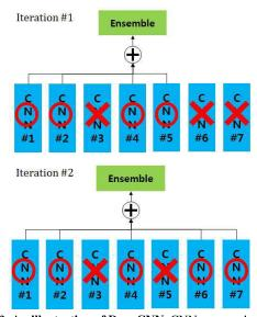
Figure 2. **An illustration of DropCNN.** CNNs are randomly chosen at each iteration during the JF training.
