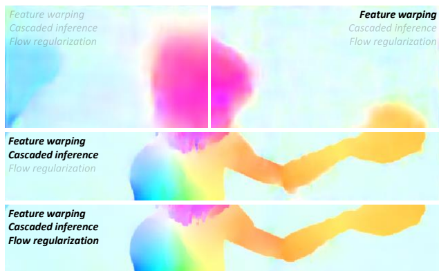
Figure 1: Examples demonstrate the effectiveness of the proposed components in LiteFlowNet for i) feature warping, ii) cascaded flow inference, and iii) flow regularization. Enabled components are indicated with bold black fonts.
