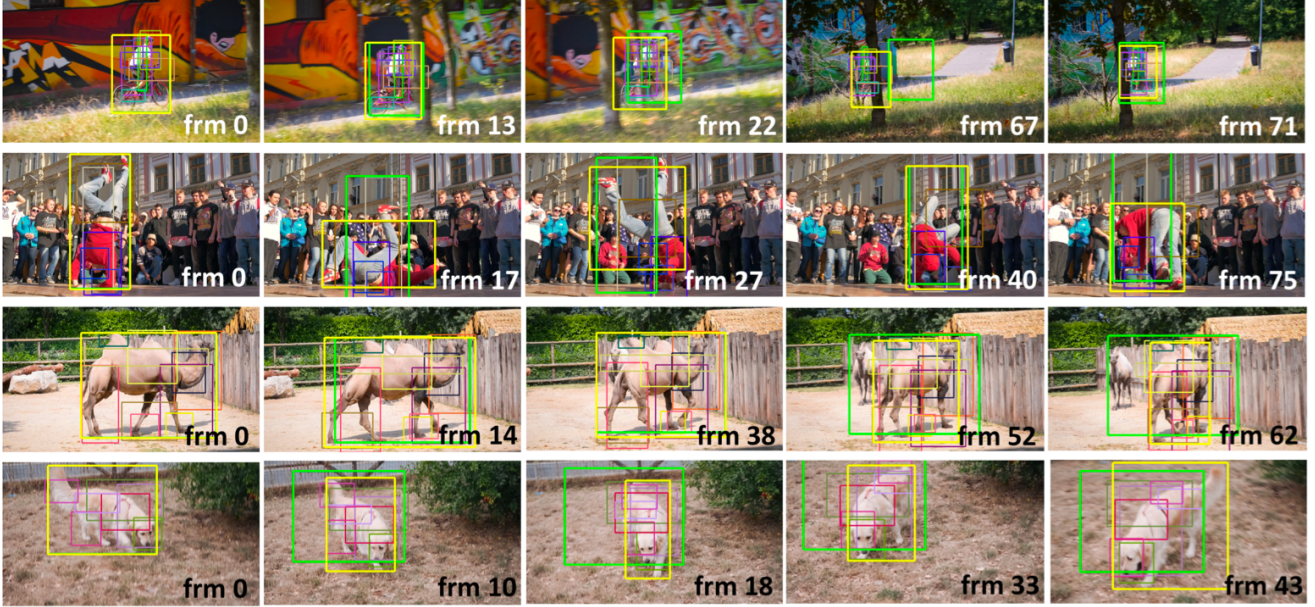
Figure 3. Sample results for part tracking. We show some high-scored parts and their tracking results. Green and yellow boxes are the results by applying object tracker [2] and by our method via aggregating parts, respectively. It shows that our result (yellow boxes) are robust to object deformation and occlusion, due to the stability of tracking parts.
