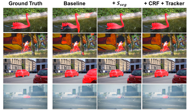
Figure 7. Sample results of using different components in the proposed method. We show gradual improvement over baseline with part aggregation, CRF refinement and an object tracker.
