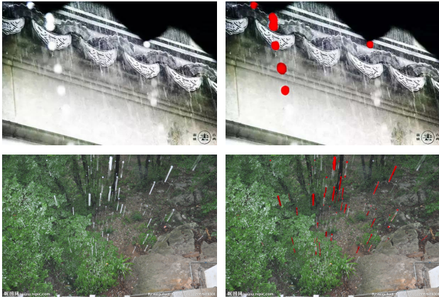
Figure 3. Examples of rain occlusions in video frames. Compared with additive rain streaks, the rain occlusions (denoted in red color) contain little structural details of the background image.
