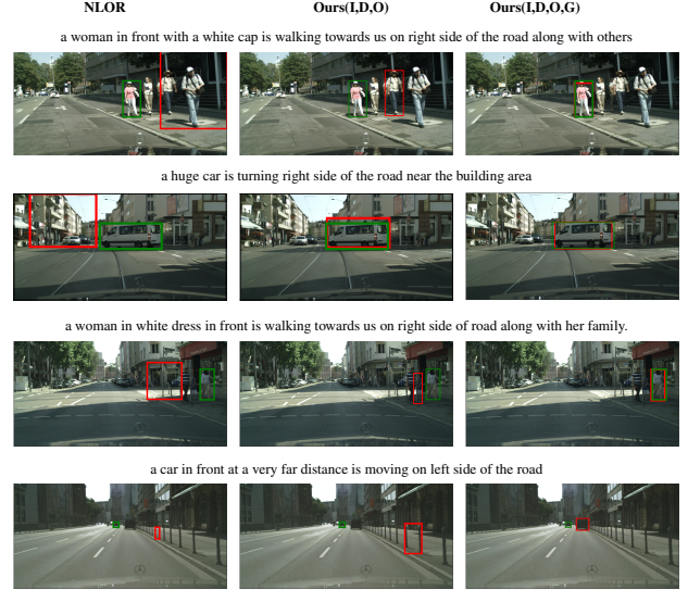
Figure 5: Some qualitative results from: NLOR (left column), Ours(I,D,O) (middle) and Ours(I,D,O,G) (right column). These results are obtained on the Cityscapes. Green : ground truth box and Red : predicted box.
