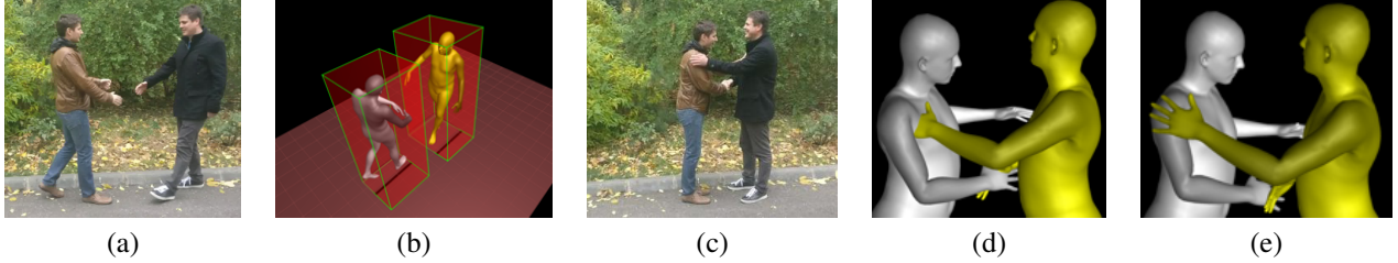
Figure 5: Adaptive volume occupancy avoidance. (a) input image where people are far apart, (b) visual representation for far-range collision check. (c) image where people are in contact. (d) inferred body shapes without and (e) with collision constraint, which ensures correct contact without simultaneous volume occupancy.
