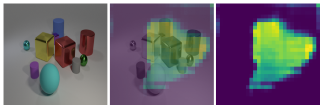
Figure 7. An input image (left) and the attention mask produced by the Relate[right] module (right) when it receives an attention on the purple cylinder. When the attention mask is overlaid atop the input image (middle), it is apparent that the attention is focused on the region to the right of the purple cylinder.
