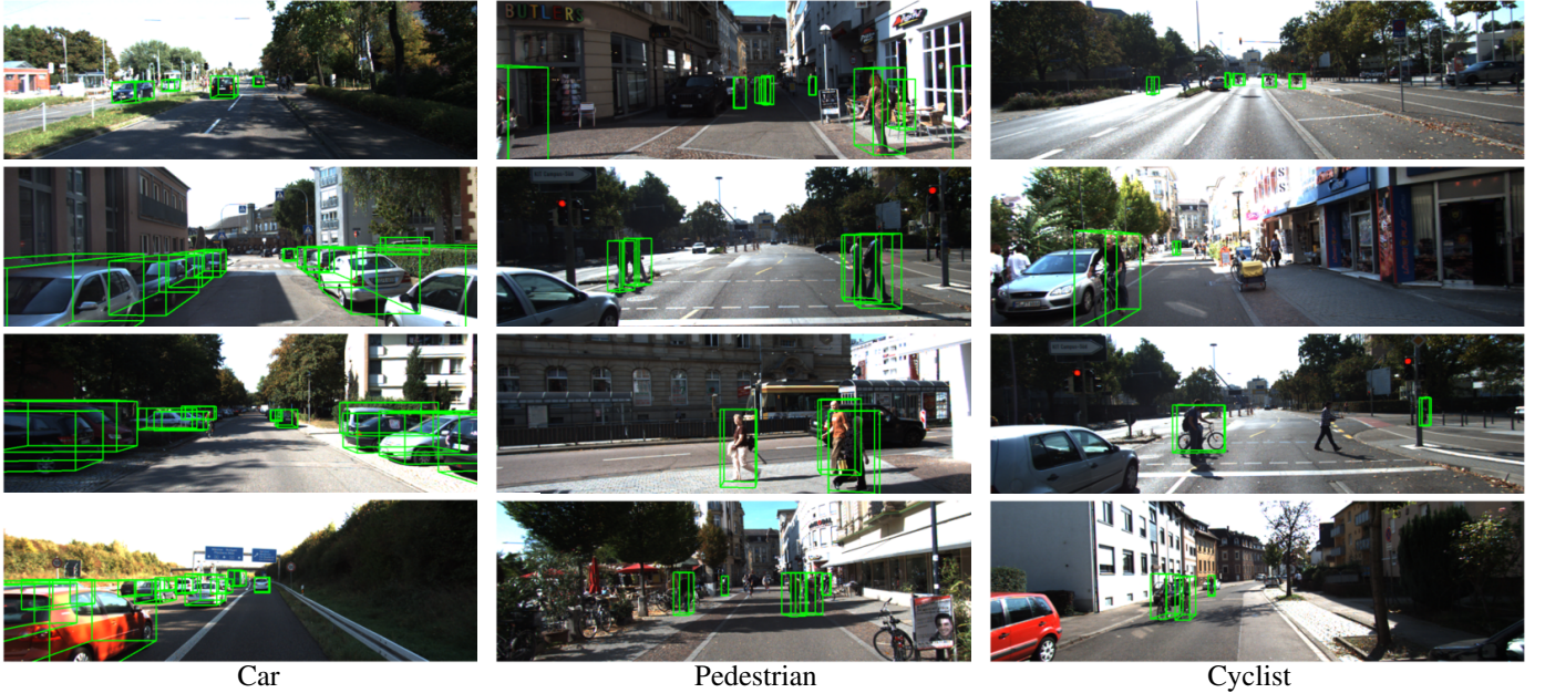
Figure 6. Qualitative results. For better visualization 3D boxes detected using LiDAR are projected on to the RGB images.
