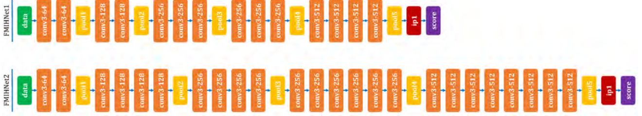
Figure 6. Network architecture: FMIHNet1 for Var and CFA features; FMIHNet2 for Grad, ADQ and NOI features.
