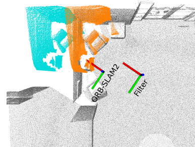
Figure 9. Comparison of registration of current sensor measurement at ground truth point cloud (gray) at ORB-SLAM2 pose estimation (cyan) and at the estimated filter pose (orange). The sensor measurement aligns with the ground truth point cloud in the filter estimate frame while the accumulated drift in the ORB-SLAM2 frame due to transition through a less feature rich region leads to poor alignment.
