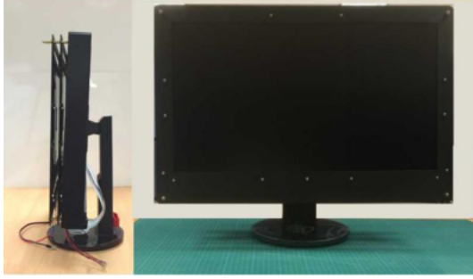
Figure 7. Hardware prototype of compressive light field display.
