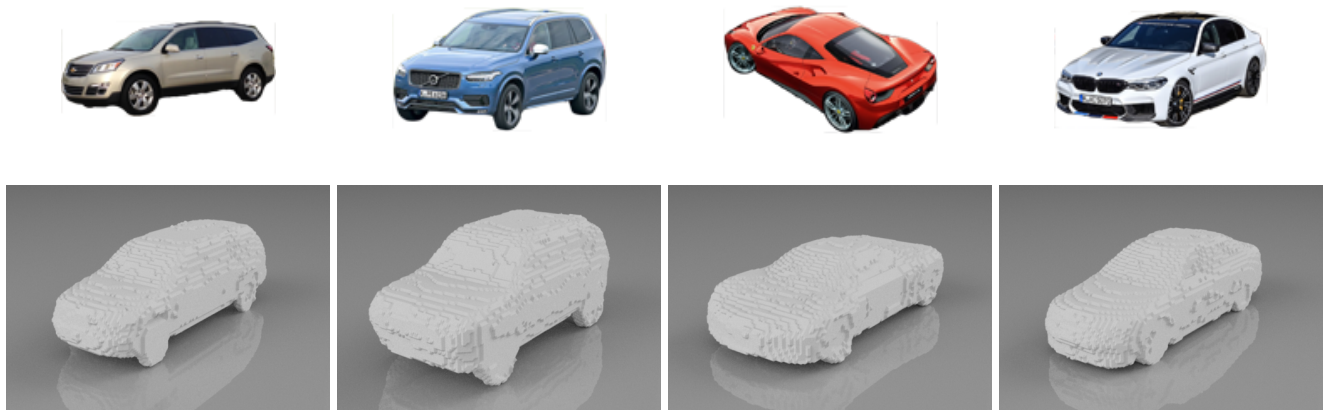
Figure 11: Qualitative results at high resolution ( 128^3 ) for real-world images of cars. For a given input image (top row), our Matryoshka network predicts a 3D shape (bottom row).
