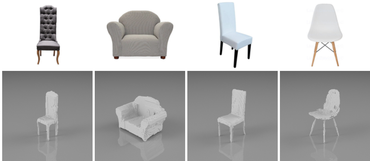
Figure 10: Qualitative results at high resolution ( 128^3 ) for real-world images of chairs. For a given input image (top row), our Matryoshka network predicts a 3D shape (bottom row).
