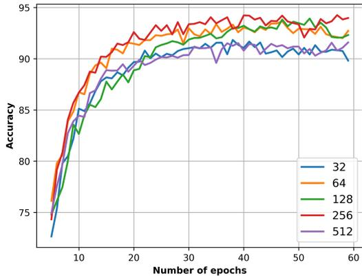
Figure 2: Effect of the noise dimension on classification accuracy for the transfer task SVHN  $\rightarrow$  MNIST
