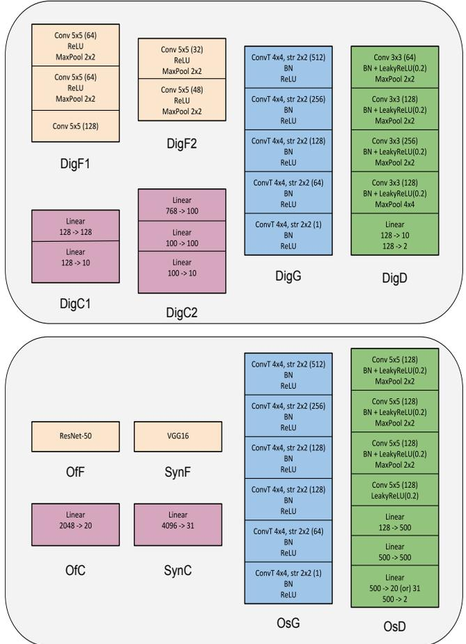
Figure 1: Network Architectures. Legend: BN - Batch Normalization, ConvT - Transposed convolution layer
