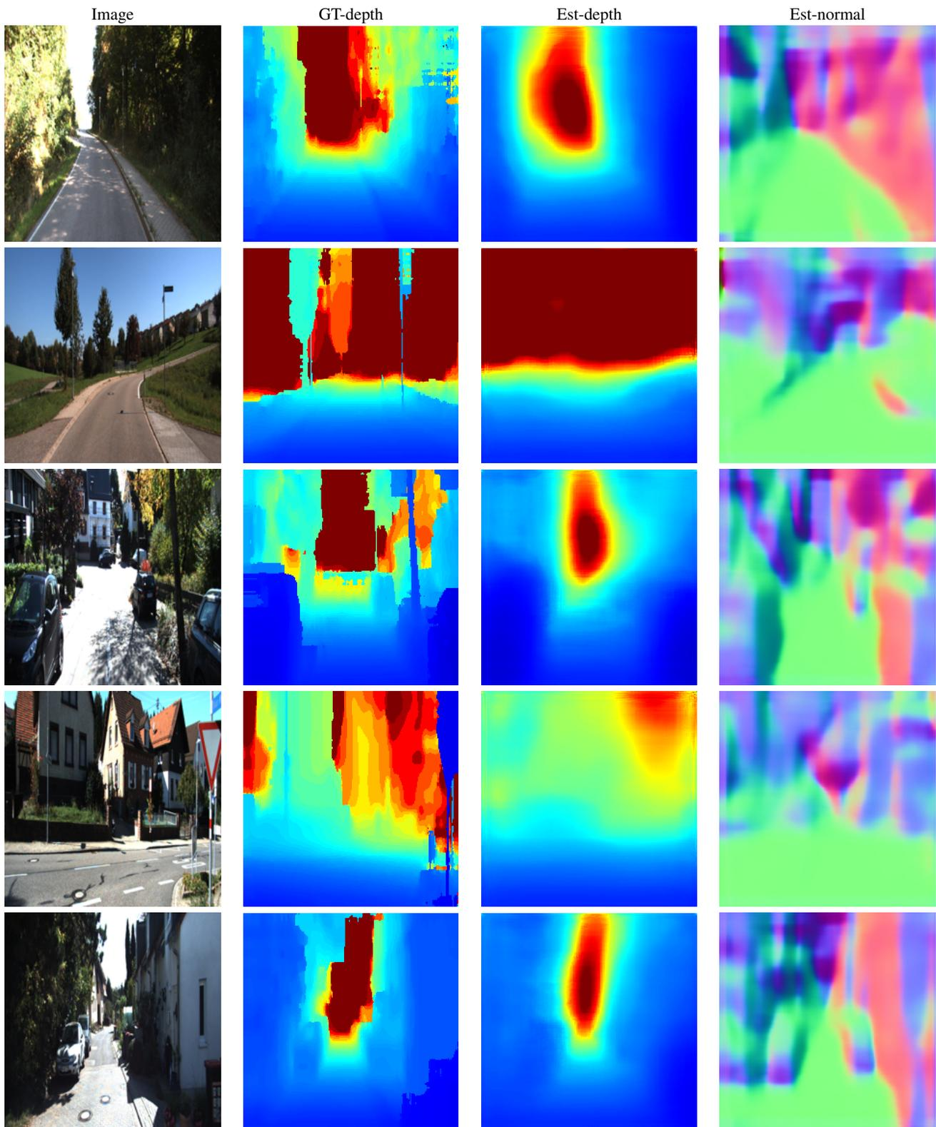
Figure 8. Visualization of the estimated depth and normal for KITTI. Color indicates depth (red is far, blue is close).
