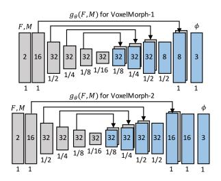
Figure 3: Proposed convolutional architectures implementing  $g_{\theta}(F,M)$ . Each rectangle represents a 3D volume. The number of channels is shown inside the rectangle, and the spatial resolution with respect to the input volume is printed underneath. VoxelMorph-2 uses a larger architecture, using one extra convolutional layer at the output resolution, and more channels for later layers.
