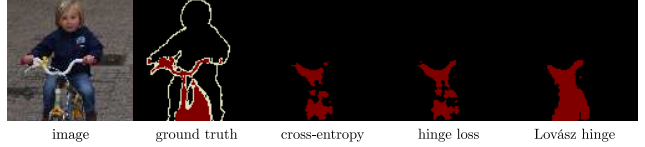
Figure 4: Binary bicycle masks predicted on a validation image after training the network under various losses.
