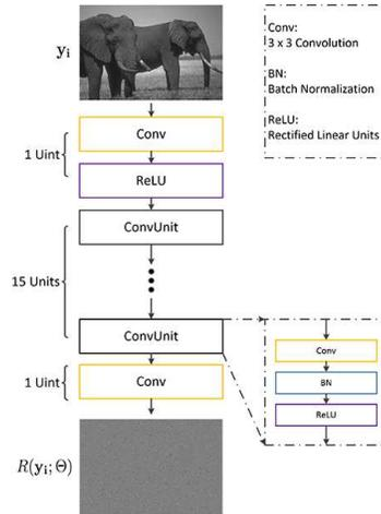
Figure 4. The network architecture of the Convolutional Neural Network. The input is a noisy image  $\mathbf{y}_i$ , and the output is the difference  $R(\mathbf{y}_i; \Theta)$  between the input and the latent clean image. The predicted clean image can be obtained by  $\mathbf{y}_i - R(\mathbf{y}_i; \Theta)$ . The filter number of the last unit is equal to the output channel number. Each of the other units contains 64 filters.
