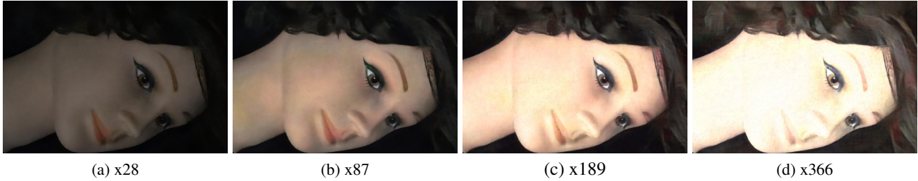
Figure 4. The effect of the amplification factor on a patch from an indoor image in the SID dataset (Sony x100 subset). The amplification factor is provided as an external input to our pipeline, akin to the ISO setting in cameras. Higher amplification factors yield brighter images. This figure shows the output of our pipeline with different amplification factors.
