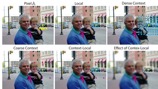
**Figure 4:** (Best viewed in color) Visualization of different feature information. The local information of pixel  $\mathbb{A}$  could not aggregate useful contexts, such as road and other cars. However, its contexts will be dominated by the features of the men in the both schemes of dense context and coarse context. The context-local scheme injects blur context to local feature of pixel  $\mathbb{A}$  to make discriminative context aware local feature.
