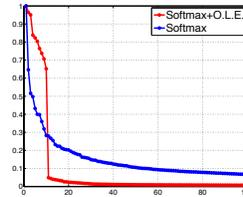
Figure 7. Spectral analysis of the deep feature matrix obtained for CIFAR10 validation data using VGG-16. We plot the normalized singular values of the feature matrix with and without OLÉ. When using OLÉ, the deep features are concentrated along 10 strong dimensions in the embedding space, corresponding to the linear subspaces where the features are compacted. For the standard softmax, the energy is distributed more evenly.
