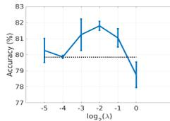
Figure 4. Validation of  $\lambda$  (11) for the STL-10+ experiment. Based on this graph, we chose  $\lambda = 0.25$  for the final training. The dotted line is the average score obtained with the standard softmax loss.
