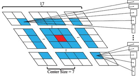
Figure 4: Illustration of center size 7 in RPN feature map, each grid represents encoded feature of  $k$  anchors at corresponding position. For example, there are  $2k$  channels representing foreground and background activations in classification feature map. The center size of anchors indicate the search region of the model.
