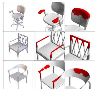
Figure 10: Different thumbnails of the same shapes (first column) created to highlight detected “armrest” (second column) and “back” (third column) regions.
