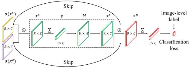
Figure 3: The network architecture of surrogator  $F$ .
