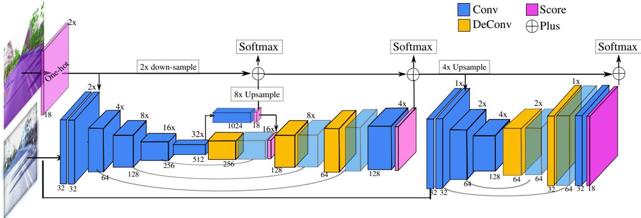
Figure 4: Architecture of the segment CNN with rendered label map as a segmentation priori. At bottom of each convolutional block, we show the filter size, and at top we mark the downsample rates of each block w.r.t. the input image size. The ‘softmax’ text box indicates the places a loss is calculated. Details are in Sec. 4.3.
