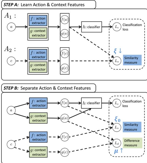
Figure 3. **Two-stage optimization of the proposed framework.** Step A: Learning action and context features for recognition task; Step B: Learning to separate action and context features using conjugate samples. The optimization procedure is further detailed in Table 1. Note that the dotted lines are only effective in the learning phase and removed at test time.
