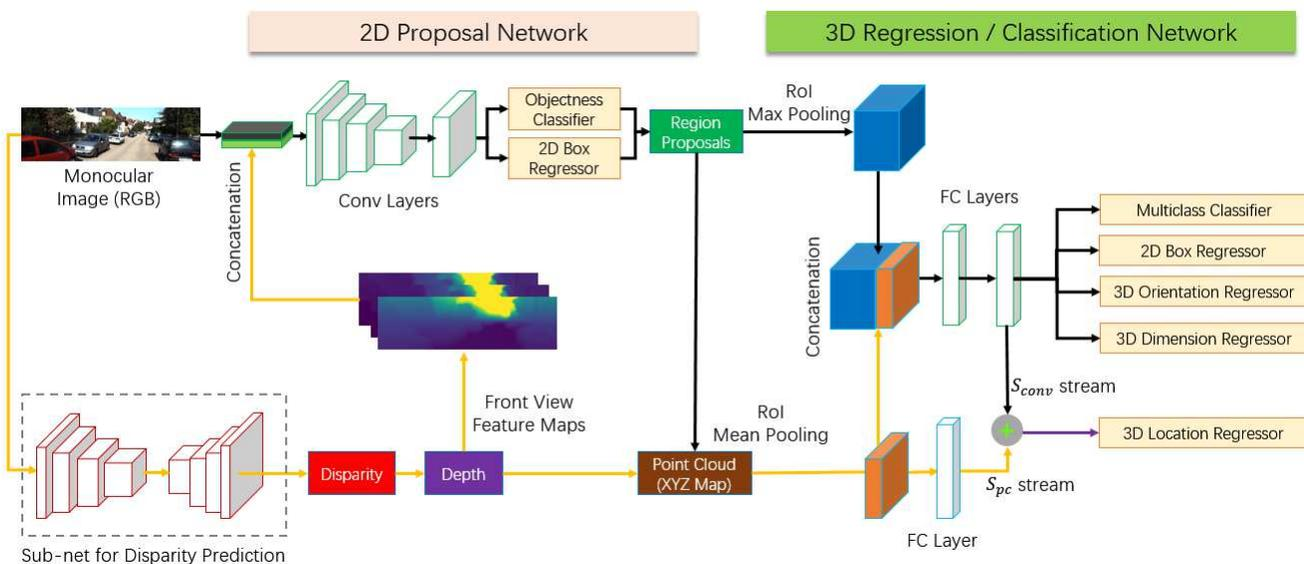
Figure 1. The proposed framework for 3D object detection.
