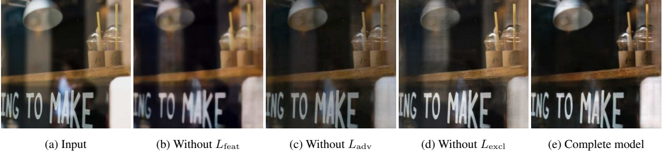
Figure 2: Visual comparisons on the three perceptual loss functions, evaluated on a real-world image. In (b), we replace L_{\text{feat}} with image space L^1 loss and observed overly-smooth output. (c) shows artifacts of color degradation and noticeable residuals without L_{\text{adv}} . In (d), the lack of L_{\text{excl}} makes the predicted transmission have undesired reflection residuals. Our complete model in (e) is able to produce better and cleaner prediction.
