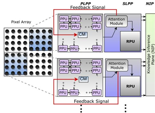
Figure 3. PPU-RPU interconnection structure with feedforward and feedback connections.
