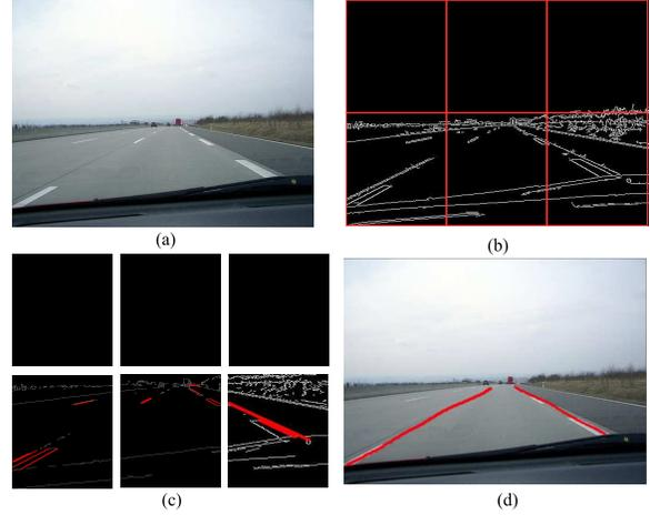
Figure 10. Images in the Hierarchical Plane, (a) Image input in the PLPP layer (b) Output of the PLPP (c) Output of the SLPP (d) Output of the NIP layer. The lanes are highlighted in the main image with red marks [28].
