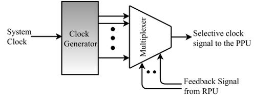
Figure 6. Clock Musk (CM) unit: *System Clock* is divided into number of clocks and feedback signal determines the appropriate clock for the Digital Processor.
