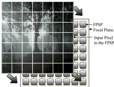
Figure 1. Focal Plane Image Processing; Each block in the image corresponds to an Focal Plane Sensor Processor.
