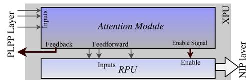
Figure 7. XPUs single flow in the SLPP: The Attention Module and RPU.
