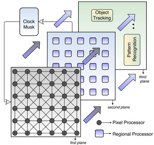
Figure 2. Overview of the 3D bottom up architecture of the smart image sensor. The computational units are organized in planes, where the output of each layer serves input for the next one.
