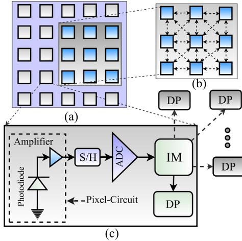
Figure 4. (a) PPU array in the PLPP layer (b) Interconnection among the PPU (c) Components of a PPU includes *Pixel Circuit*, *ADC*, *Interconnect Manager*, and *Digital Processor*.
