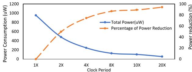
Figure 9. Power Consumption versus time period analysis in the DP: The 10 times slower clock has 89% power savings.
