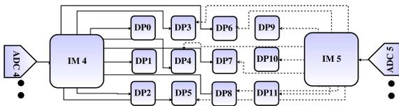
Figure 5. Signal flow from the ADC to Digital Processors(DP): *ADC-4* is connected to *DP-4* and its neighbor, and similarly *ADC-5* is connected to *DP-5* and its neighbor.
