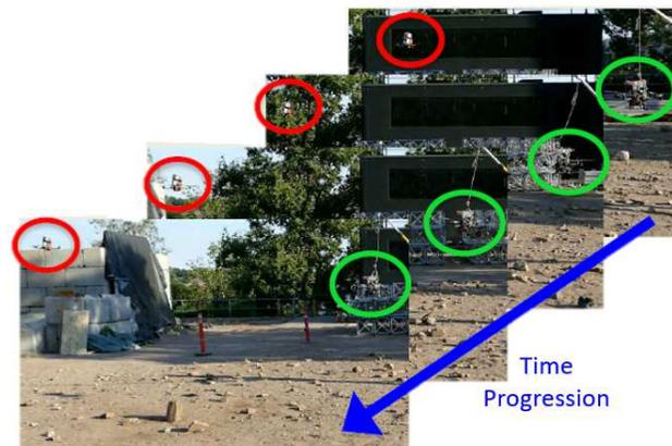
Figure 1: Follower drone (green) autonomously tracks a manually joy-sticked leader drone (red)
