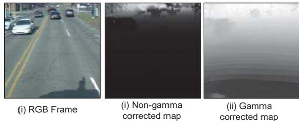
Figure 4. Gamma correction on the LiDAR depth map amplifies darker regions to bring out more details.
