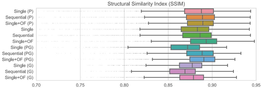
Figure 6. Box plot of the SSIM visualizing the distribution of reconstruction error for each frame in the FORD test set. *P* indicates that the dataset has been *pruned* to remove stationary data as opposed to using the full dataset. *G* indicates that the depth map has been gamma corrected. *PG* means that both processing techniques have been applied. The abbreviation *OF* means optical flow. Higher scores are better. An SSIM of 1 is the highest possible score indicating perfect reconstruction.
