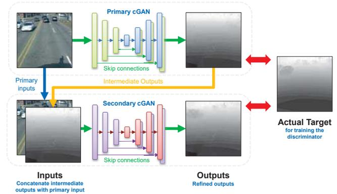
Figure 2. An illustration of cascaded refinement by training multiple GANs in stages. The first stage produces a coarse estimate of the depth map, while the second stage refines the first estimate by processing a fused version of it with the original inputs.
