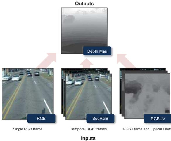
Figure 1. Three formulations of the task at hand. We estimate the depth map of a scene using individual frames (left), sequential frames (center), and optical flow (right) from the video data and attempt to estimate the depth map of the scene as the output. Note that each image frame contains three color channels.
