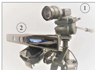
**Figure 2:** The Physiological Camera in real-time system (PhysC<sub>RT</sub>): 1) Digital Color Video Camera, 2) Microsoft Kinect.
