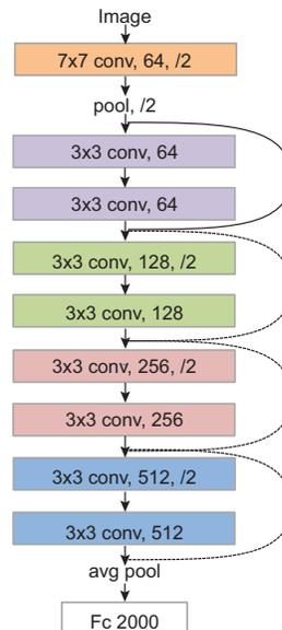
Figure 2. 10-layer ResNet Architecture
