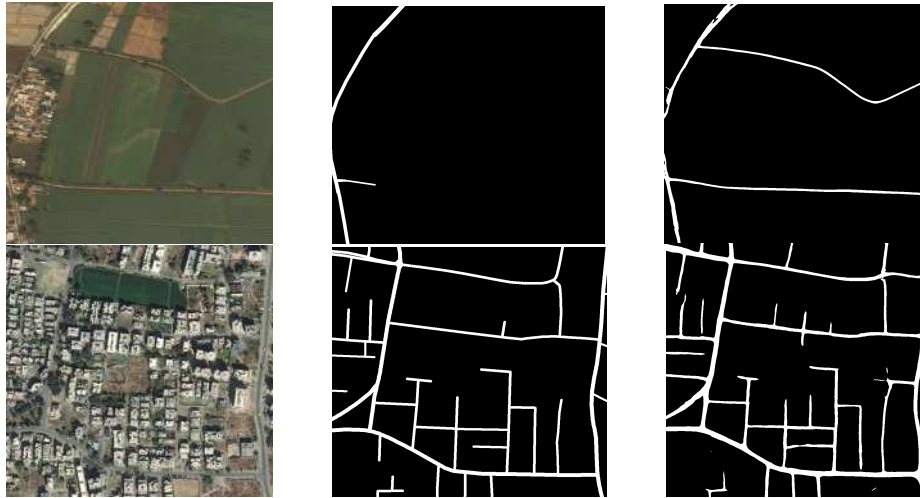
Figure 2: Examples for NU-Net Road Extraction results versus true masks. First column has the original images, second column has the true masks and third column has NU-Net predictions.
