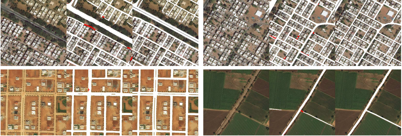
Figure 9. Illustration of prediction and post-processing. The three figures in a row are the satellite image, the prediction output with post-processing add-on in red, and the ground truth.
