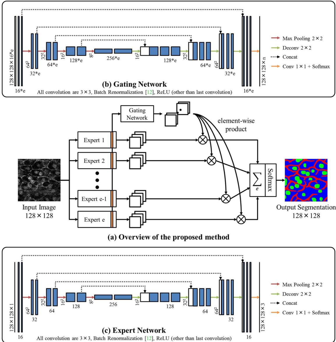
Figure 3. (a) Overview of the proposed method. (b) The detail of Gating network. (c) The detail of Expert network.  $e$  indicates the number of Expert networks. In this paper, we set the number of initial filters of Expert network as 16.
