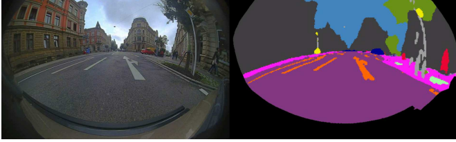
Figure 7: Semantic Segmentation on a fisheye automotive camera
