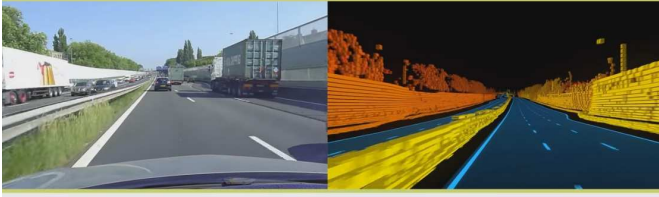
Figure 4: Example of High Definition (HD) map from TomTom RoadDNA (Reproduced with permission of the copyright owner)
