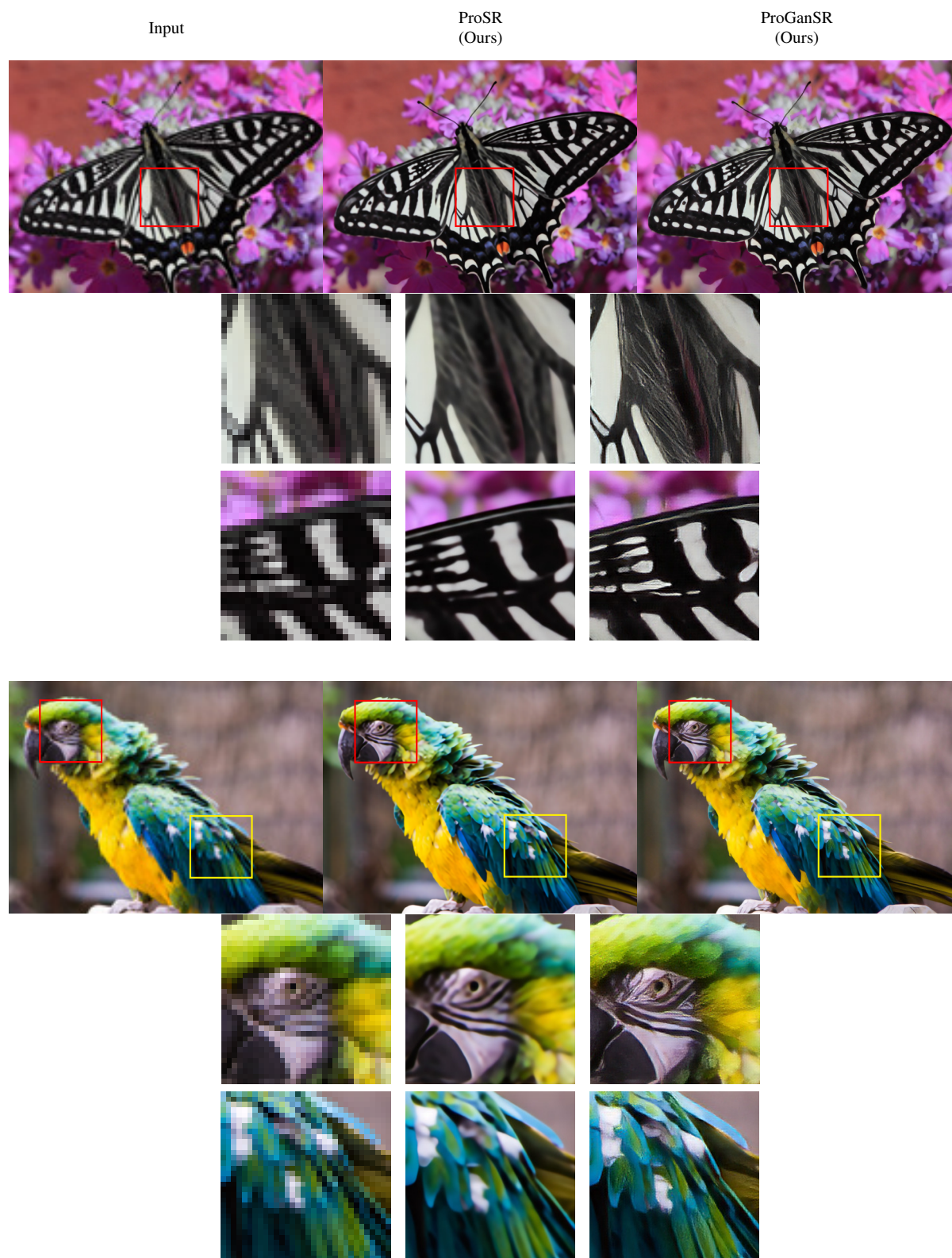
Figure 1: 8\times ProGanSR results compared to ProSR.
