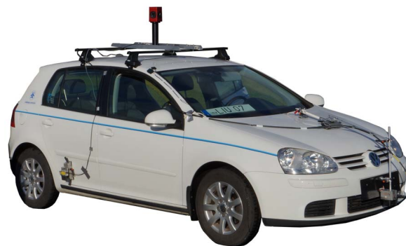
Figure 1. Test platform car with roof rack mounted Ladybug 3
