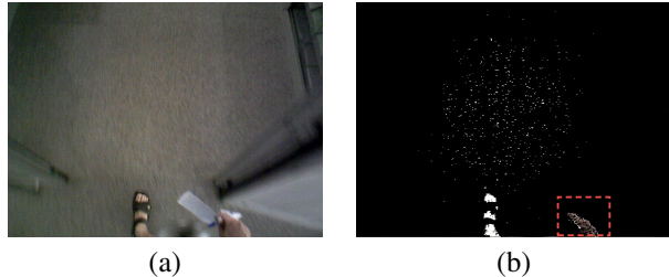
Figure 2. Skin segmentation. (a) Original raw image (b) Segmentation using color and depth filtering. The white pixels (those that are NOT within the dashed rectangle) were accepted by the color filter but rejected by the depth filter. Depth helps us to filter out feet and ground reflection pixels within the skin color range.
