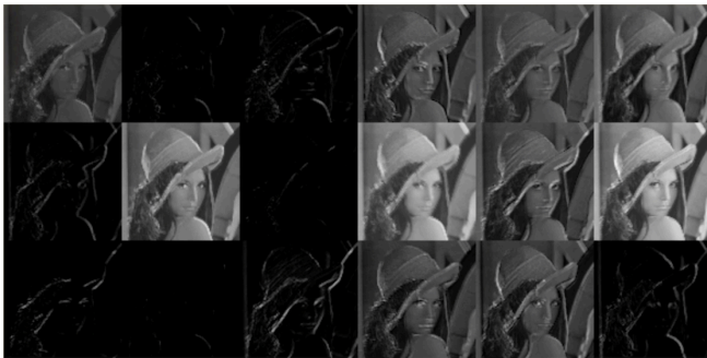
Figure 3: Single neural network layer with 4 input planes of 500 \times 500 , 18 outputs planes and 3.6 billion operations per frame. nn-X computed one frame in 6.2 ms and was 271 times faster than the embedded processors.
