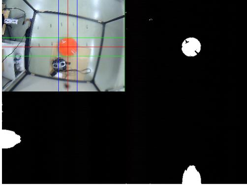
Figure 6. Debug output of the FPGA. The correct acquisition of the target position and size and the histograms are shown.
