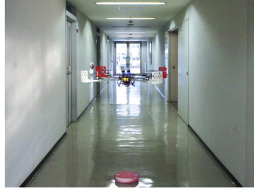
Figure 8. Successful test of the hold position and altitude task in a corridor
