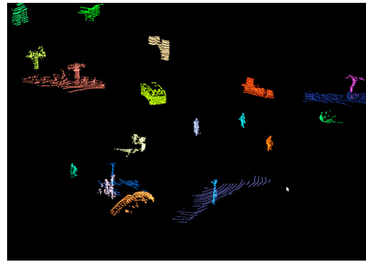
Figure 6. An example of 3D blobs obtained with the clustering-based approach applied to the point cloud without ground plane. Colors are mapped to segmented blob IDs.
