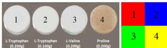
Figure 4. An image of four chemical compounds in visible spectrum in the left and the ground truth of the THz image in the right.
