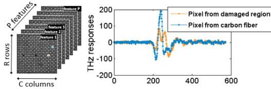
Figure 1. In the left, 3D THz data cube represented by  $R \times C$  pixels and characterized by  $P$  raw features. The two pixels colored in blue and orange, which belong respectively to a typical region of the carbon fiber and a damaged zone, correspond to the two THz responses with the same colors in the right.
