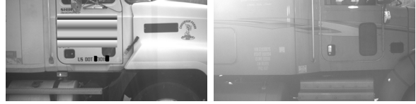
Figure 1. USDOT image samples with high contrast (a) and low contrast (b) acquired by an NIR camera.
