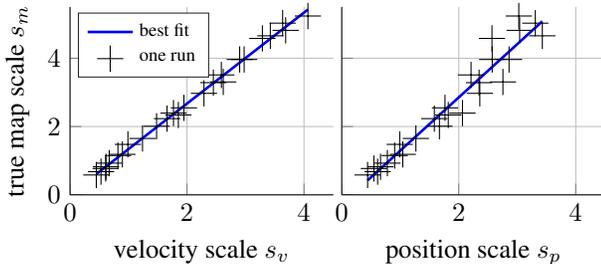
Figure 3: Linear dependency between UKF-estimated scales and the true map scale. Velocity and position scale have the same ground truth.
