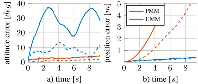
Figure 4: Error-time dependency for pose estimation without visual update. Dashed lines indicate the standard deviation.
